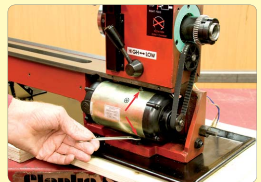
40. Slacken the two drive belt adjusting screws.
