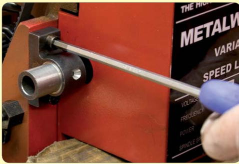
109. Loosely fit leadscrew bracket & grease bore.
