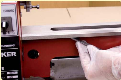
84. Scrape any paint off the bed shears.
