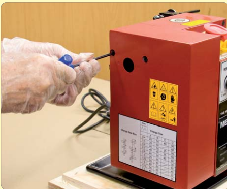
18. Remove the gear cover.
