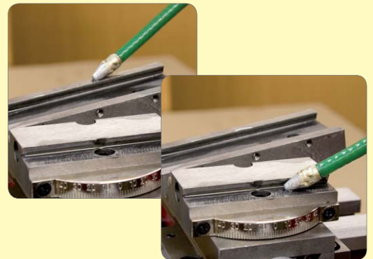
168. Oil top slide assembly and fit.
