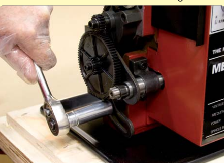
20. Undo and remove the gear quadrant.
