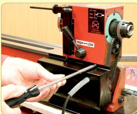
39. Remove the motor cover.
