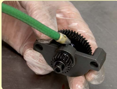
124. Oil gear shaft.
