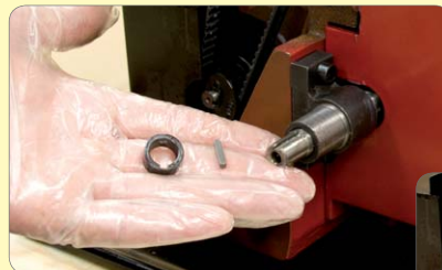
24. Remove the spacer and key from the main leadscrew.
