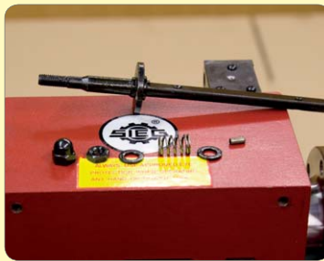
80. Refit the chuck guard assembly.
