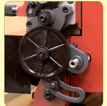
131. Refit lower gear quadrant.
