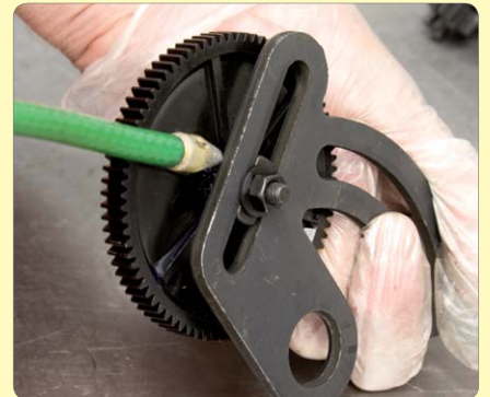
125. Oil the lower quadrant gear shaft.
