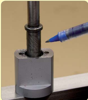
154. Grease / oil the feed screw and bracket.
