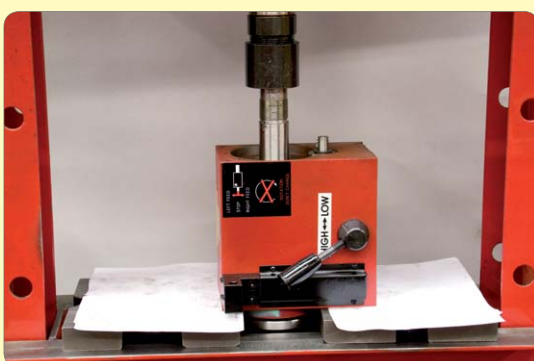
51. Press spindle out of head.
