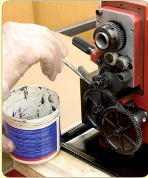
137. Very lightly grease gears.
