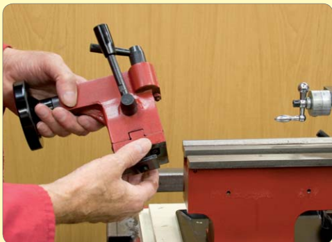
3. Remove the tailstock.
