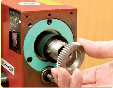
46. Remove Spindle Gear.
