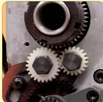
129. Check neutral gear position.
