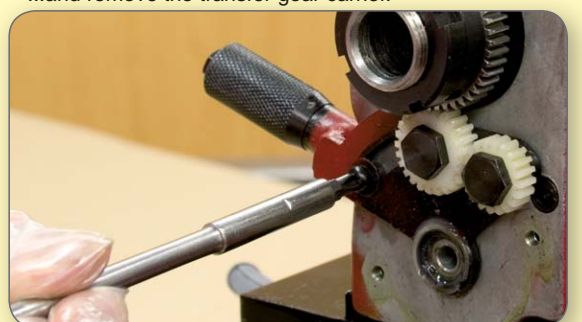
22. Undo and remove the tumbler reverse arm.
