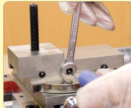
177. Final adjust the top slide gib to your preference and lock-off the screws.
