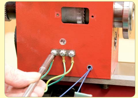
34. Disconnect the three earth wires.
