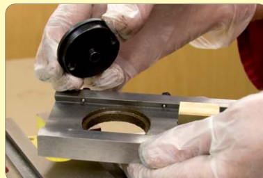
150. Fit top slide base retaining plate.
