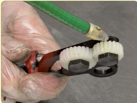
123. Oil the tumbler reverse gear shafts.
