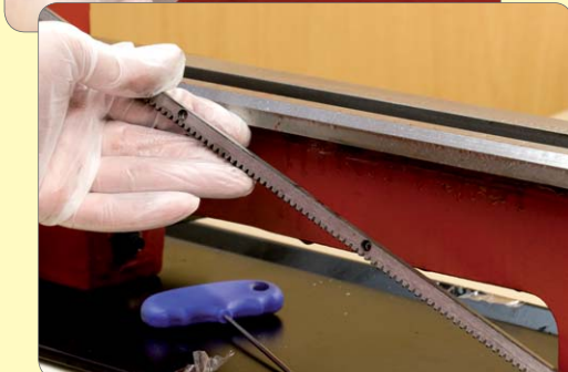
30. Remove the rack from the front of the bed.
