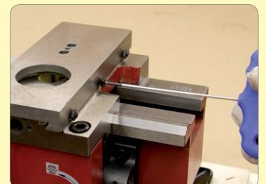
148. Fit adjusting screws lightly.
