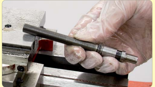
9. Slacken the gib adjusting screws.
