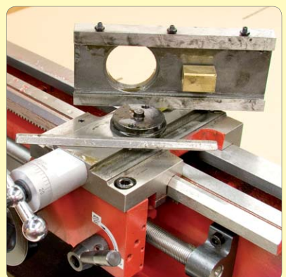
14. Slacken the gib adjusting screws.
