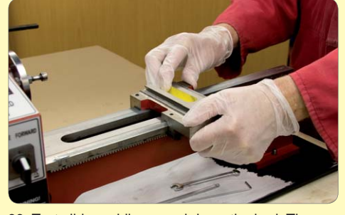
99. Test slide saddle up and down the bed. There should be slight drag with no free play. Lightly pinch up remaining cap screws checking after each one and adjusting as required.
