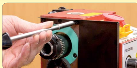
31. Remove the gear cover support bracket.
