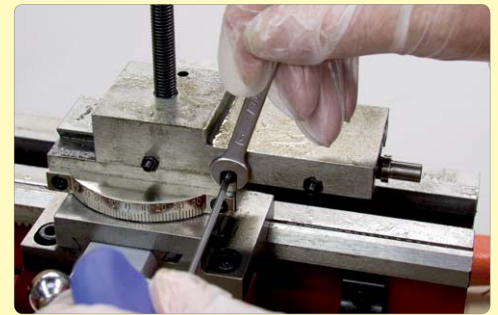
9. Slacken the gib adjusting screws.
