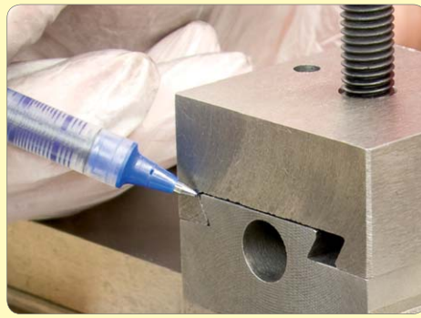
167. Temporarily fit top slide to compound base and check for clearance in corners of dovetail.
