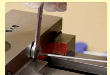
163. Make final adjustments to the gib screws for free movement of the handle with little drag.
