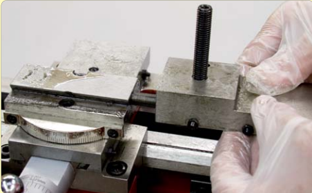
10. Remove compound slide and gib strip.
