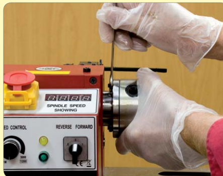
4. Remove the chuck.
