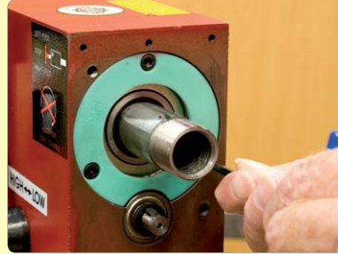
48. Remove the spindle rear bearing cover.
