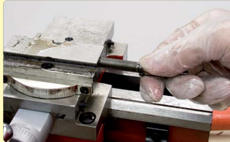
11. Unscrew the leadscrew from the compound slide base.
