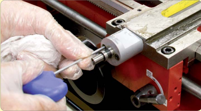
17. Remove the leadscrew end plate and leadscrew.
