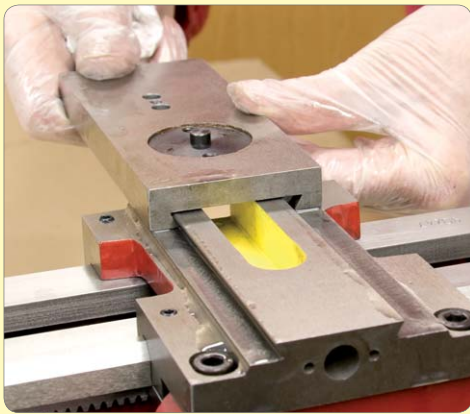
152. Assemble onto saddle.
