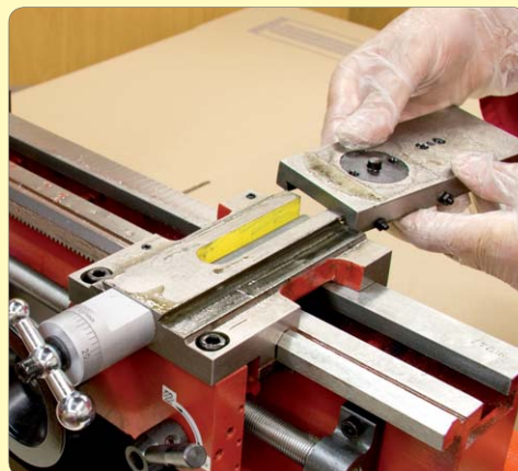
15. Pull off the cross slide assembly.
