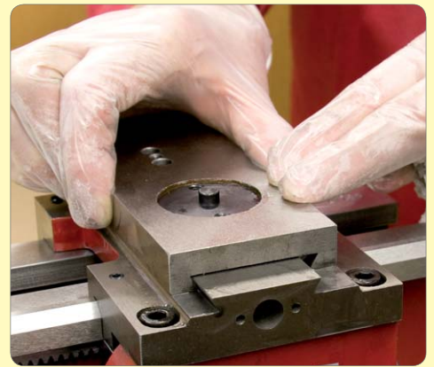
153. Fit adjusting screws and adjust so slide can be moved back and forth easily by hand.
