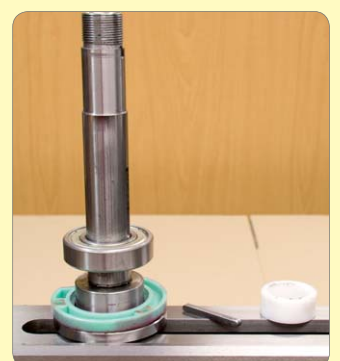
52. Remove spacer and key.
