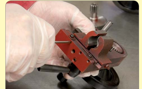
102. Adjust the gib screws if necessary.
