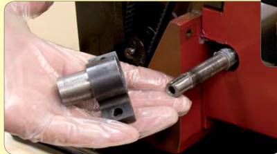
24. Remove the spacer and key from the main leadscrew.
