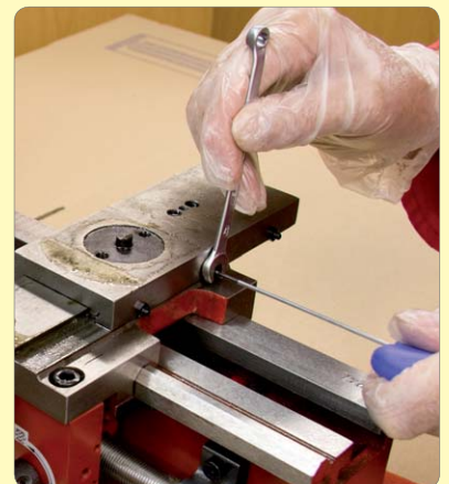
14. Slacken the gib adjusting screws.
