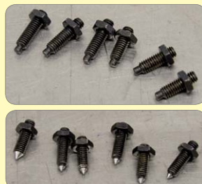
146. Modify gib screws or replace with cone point screws.
