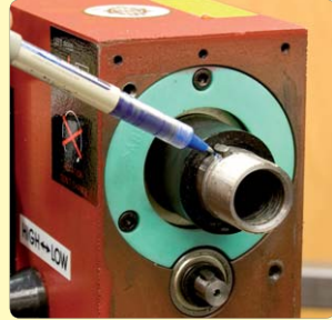
47. Remove key and spacer.
