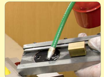
148. Fit adjusting screws lightly.
