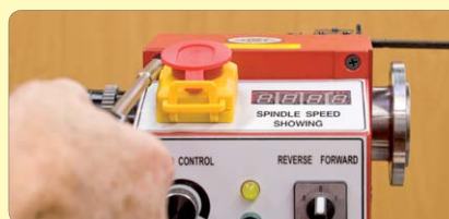
32. Remove 4 screws securing the control panel and lay to one side.
