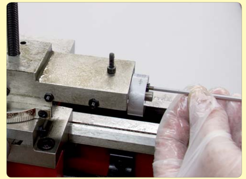
8. Remove the leadscrew end plate.
