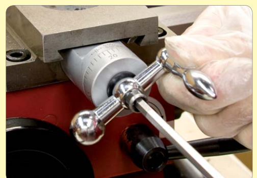
165. Refit the handle assembly.
