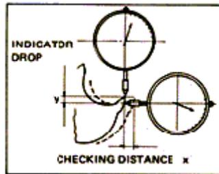
3. Roll the cutter the tabulated amount given under "checking distance" using the second indicator as a control.
