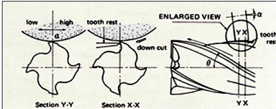
If the cutting edge of the end mill is advanced, in the helixed axial direction, being supported by the wheel transverse the points (a), (b), (c), (d), (e). The curved line connecting the point (a), (b), (c), (d), (e) is the tangent line of eccentric relief. As Figure (see) the point (e) is ground to be lower than the point (a), and the point (e) and the point (a') are positioned concentric.
