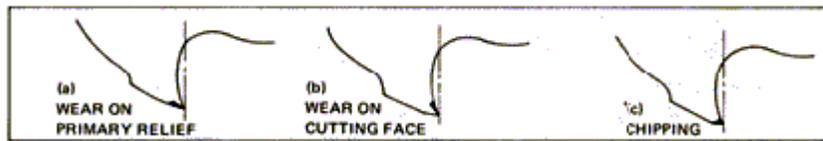
The wear on primary land is seen often. And sharpening the primary land makes the end mill perform almost the same as new one. The width of the wear land develops very fast after a time period of use, resulting in rough surface finish and chipping. Resharpener must be done before it occurs. In general, when the width of wear land become 0.2 - 0.4 mm (in case of roughing end mill: 0.5 mm) resharpener is required.
