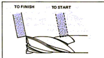
6. Checking eccentric relief & adjustment of height of tooth rest
