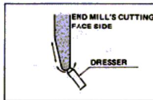
3. Angle of wheel inclination
