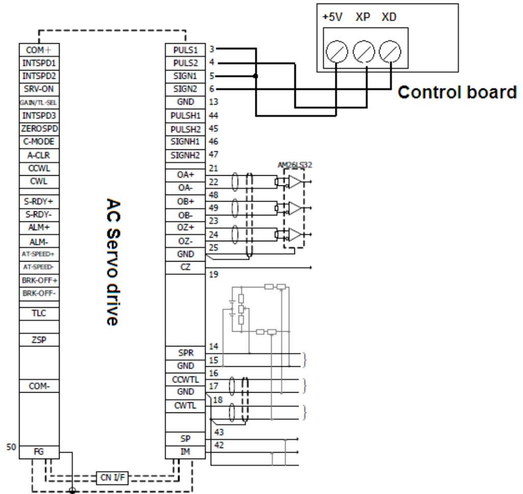
When using the AC servo driver, the control of the AC servo driver should be set as the way of pulse+direction
