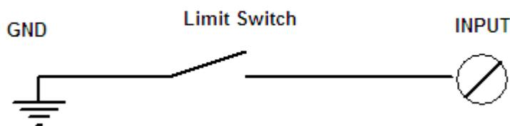
The connection diagram of the NPN style closed switch.
