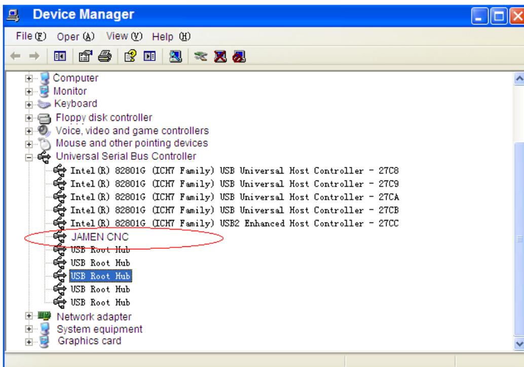
7. If the driver is not well installed, there will be a yellow question mark in front of the icon of the current device. Use the mouse to aim at the icon, click the right button, point the button of "updating the driver". Reinstall the driver, operate the software of Mach3 after the installation of the driver and the control software.
