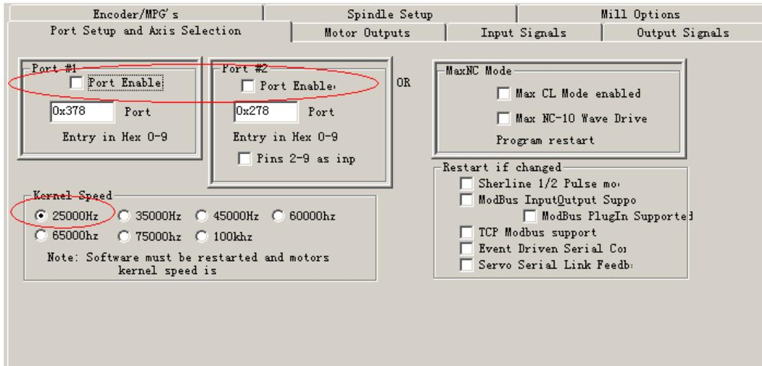
Because it is the output of the motion control card, and the parallel port is no longer used. Both of the application of the two ports are no longer used. Auto select the "100KHZ" or "300KHZ" as the core speed.
