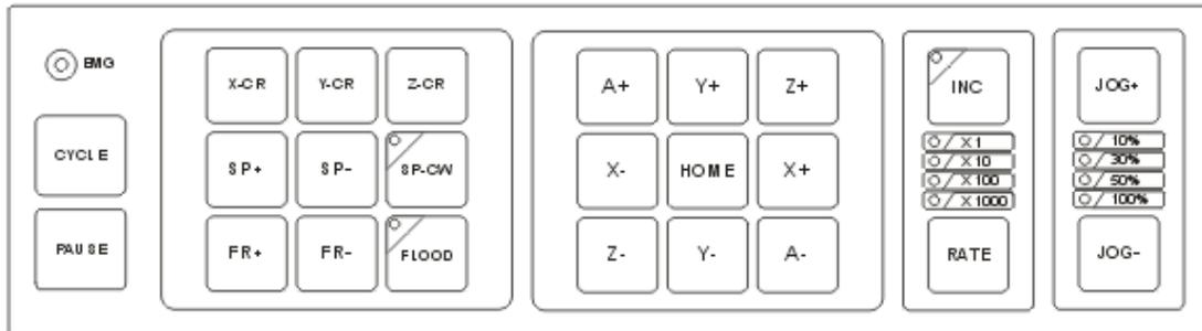
This operating board can be plugged in IDC5 socket. The initial parameters of software installation are compatible with this board. This operating board is cute and easy to use. It is convenience when you check knife and set up components axle.
