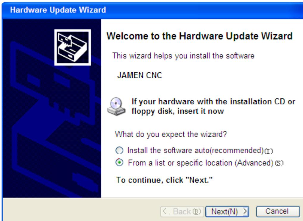
Choose the button of "instal from the list or the designated place" to continue to the next step according to the notes. The button of "instal the software automatically" cannot be selected. Press the button of "browse" in the following dialogue box, and choose the installation path for the software Mach3.
