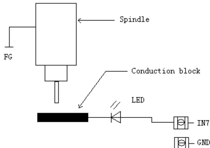
This method is in the case that the machine tool has the reliable ground connection, if we use the red pen of the universal meter to connect with +24V, and the black pen connects with frame, the machine tool is connected with the ground if there is the display of the voltage (12V-24V) .(Notes: please use the voltage grade).
