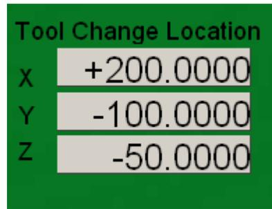
Note that the height of the number of Z axis will be of 5 to 10MM high than that of the tool setting. Such as that your connection side of the tool setting is Z - 68.000 mm, then the place of the knife changing of the Z direction is Z - 63.000 mm. After the setting of the tool setting, we can input "M900" in the input box of "MDI" in the page of "Program", and press the button of return for performing. Please choose the number of the knife before, just as the following figure:
