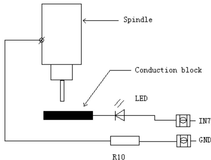
This method is to undertake the wire connection in the absolute insulation of the machine tool, and the absolute insulation refers to that the machine tool itself will not form the circuit of the power, including the existence of the leakage of the voltage. If we use the red pen of the universal meter to connect with +24V, and the black pen to connect with the frame, the machine tool is insulated if there is no display of the
