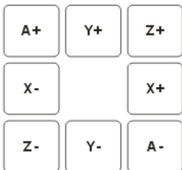
Feed shaft activate button, the corresponding axle will move when press different button; and it will stop when stop pressing. Activate speed can be adjust by pressing “JOG+” “JOG-”.
