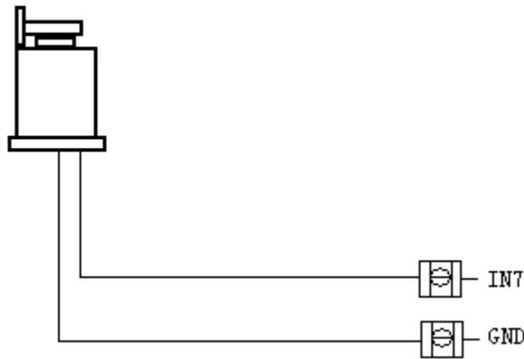
This method is the wire connection with the switch tool setting. “IN7” and “GND” must connect with the touching switch of the tool setting, and the switch must be normally open. When the tool setting is the type of Hall photoelectricity, connect the application energy with the input terminal of “IN7”, and choose the switch of the Hall photoelectricity as the type of NPN. In addition, the switch of the procedure of the tool setting may be in series connection with jerk switch.
