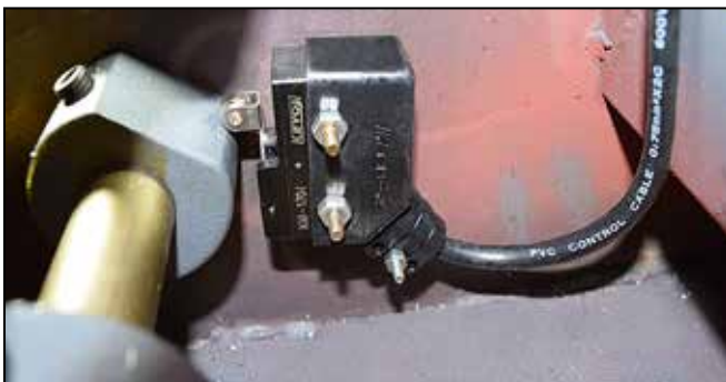
Figure 1-5 Footbrake interlock switches
