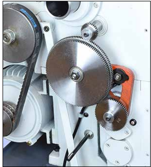
Figure 3-18 External change gears
