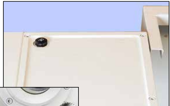
Figure 4-1 Headstock fill plug
