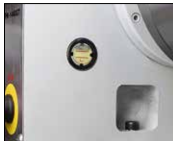
Figure 4-3 Headstock sight glass
