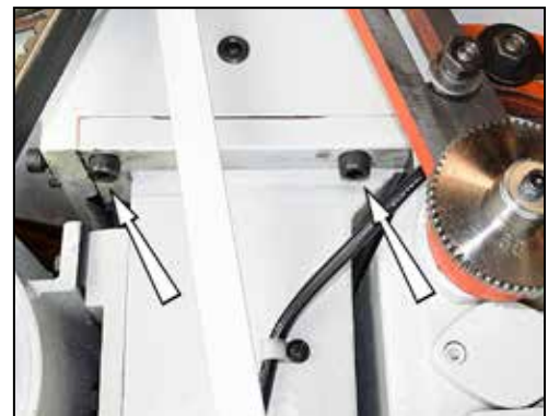
Figure A3 Headstock attachment screws, LH
