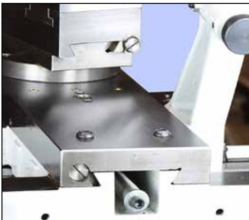
Figure 4-11 Cross slide & compound back gib screws
