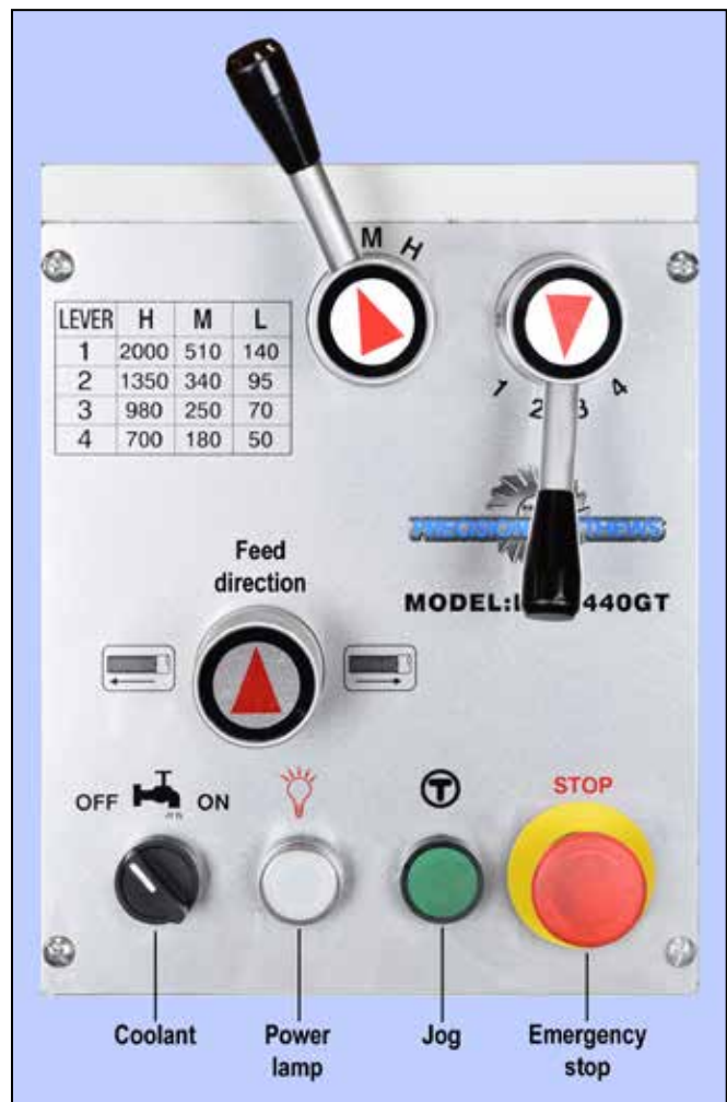
Figure 1-8 Front panel controls The Feed Direction knob is shown here in the neutral condition (no feed), leadscrew and feed shaft disengaged.
