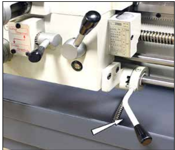
Figure 1-7 Motor control lever Mid-travel OFF, DOWN Forward, UP Reverse
