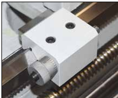
Figure 3-13 Saddle stop
