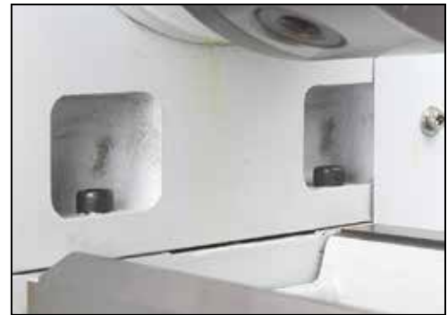
Figure A2 Headstock attachment screws, RH
