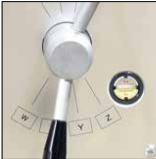
Figure 4-5 Saddle feed gearbox sight glass
