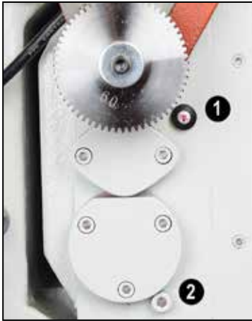
Figure 4-4 Saddle feed gearbox drain & fill plugs
