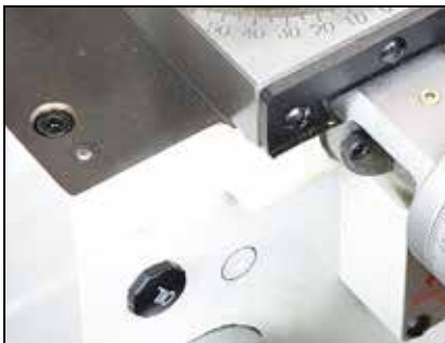
Figure 4-6 Apron gearbox fill plug
