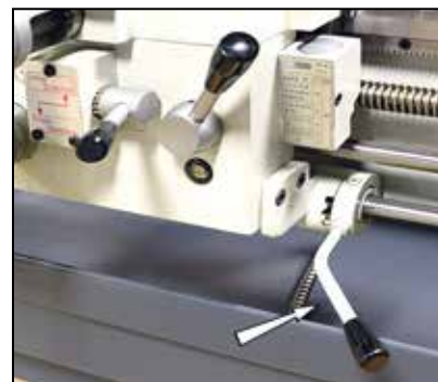
Figure 3-2 Motor control lever Mid-travel OFF, Down FORWARD, Up REVERSE
