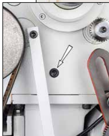
Figure 4-2 Headstock drain plug
