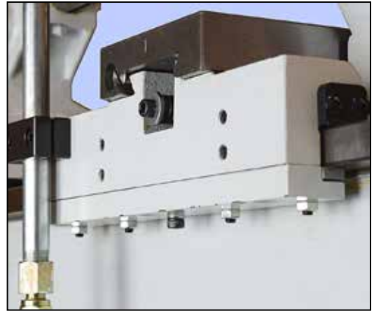
Figure 4-12 Saddle gib assembly
