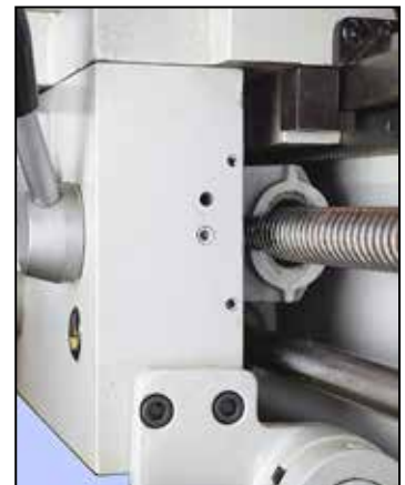
Figure 4-15 Split nut gib screws
