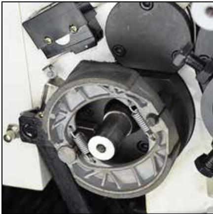
Figure 4-16 Brake assembly (representative)
