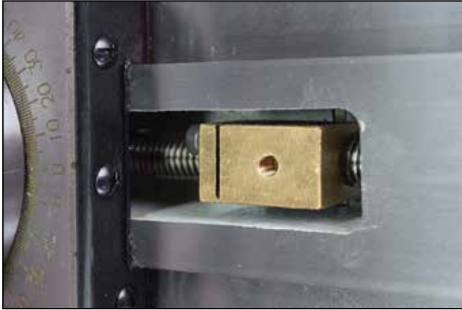
Figure 3-31 Cross slide leadscrew nut
