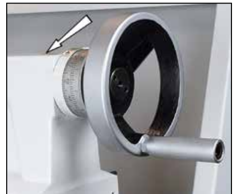
Figure 4-9 Tailstock oiler
