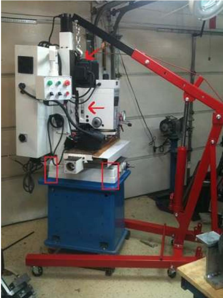
The user may wish to use a leveling base or shock absorption levelers on the base. The unit should be leveled carefully but, high precision leveling is not entirely necessary.
