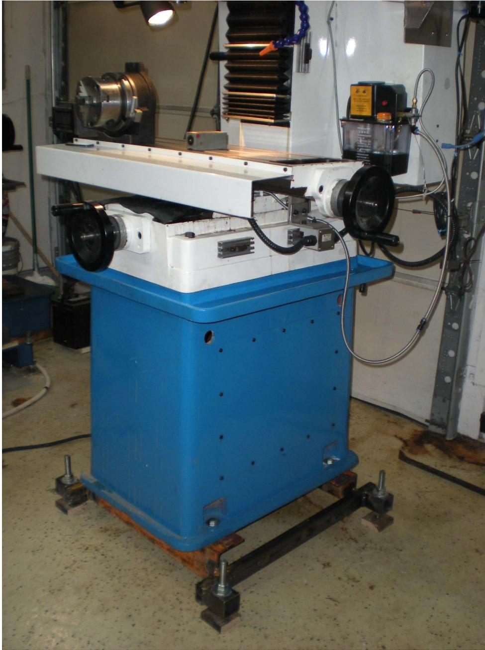
**WARNING:** During CNC operation of the mill the hand cranks will spin with significant force and possibly cause bodily injury. The protruding handle or the entire hand crank on all axis should be removed during CNC operation of the mill.
