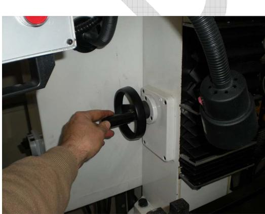
The X axis motor drive must be mounted to the table. The 4 screws and washers to attach the motor are located inside the mill table pocket. The protective paper on the mill table will need to be removed to locate the fasteners.
