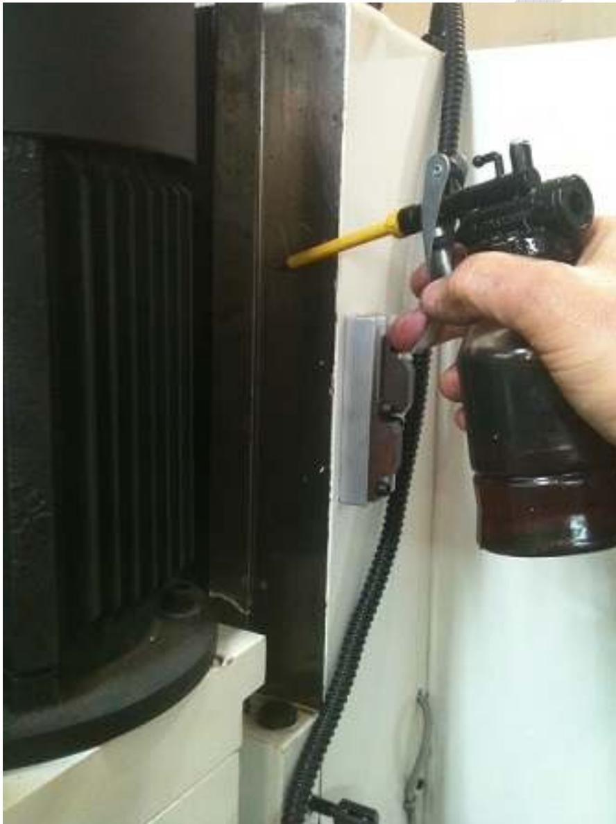
The vertical ways are not lubricated by the automatic lubrication system. The oil caps must be filled with “way”. Check the caps frequently and always refill at the start of each use. If the head position is not frequently raised up/down with more than 6” of travel, the top of the ways must be lubricated frequently as shown in the prior photo.
