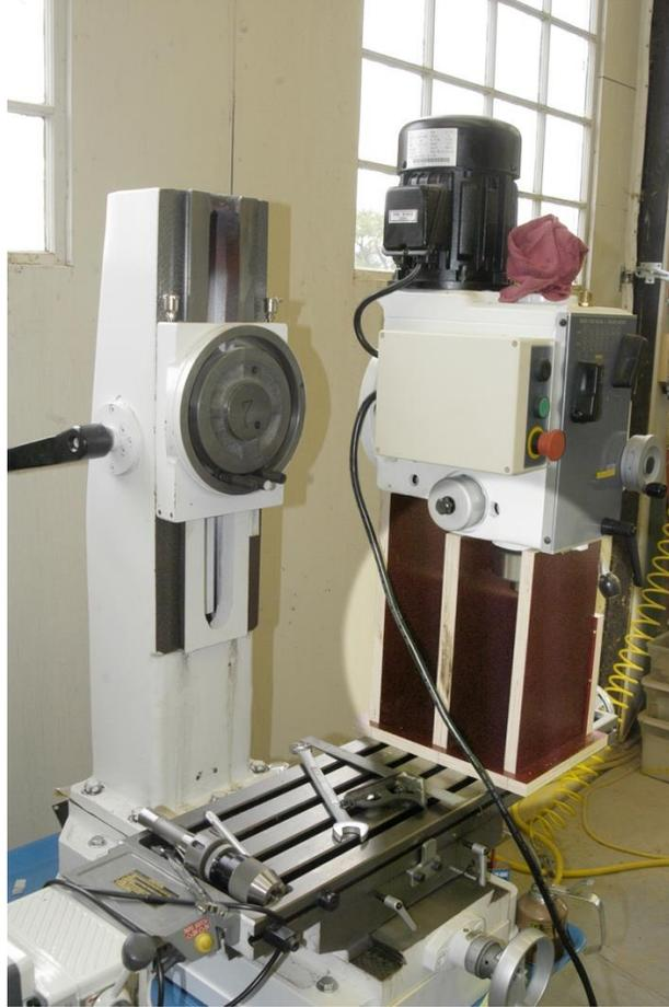
2. Remove the bolts that secure the column to the machine base, break the seal, clean up the mating surfaces and the fasteners. On some square-column mills, the bolts are easily accessed from above the machine, while on some mills, the bolts can only be accessed from under the main machine base.
