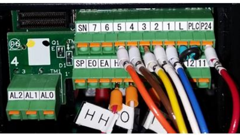
Wiring sample of control logic terminal (source logic)
