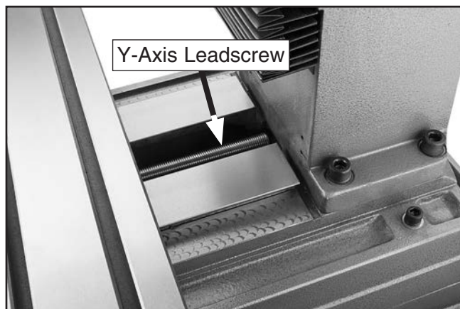
Figure 50. Y-axis leadscrew.
