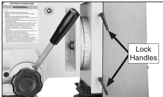
Figure 13. Lock handles for headstock elevation.
