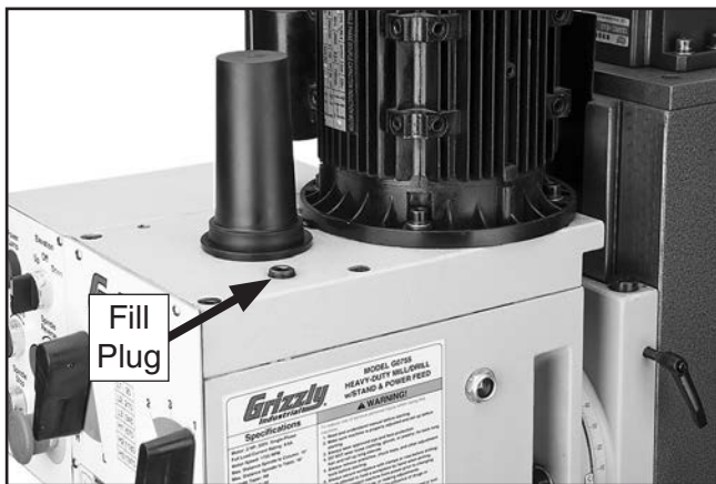
Figure 43. Headstock oil fill plug.
