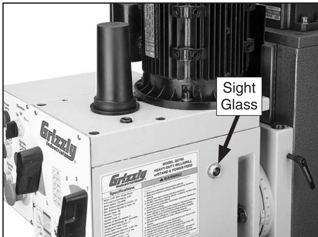
Figure 42. Headstock sight glass.
