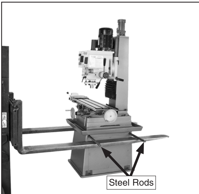
Figure 5. Lifting setup.
