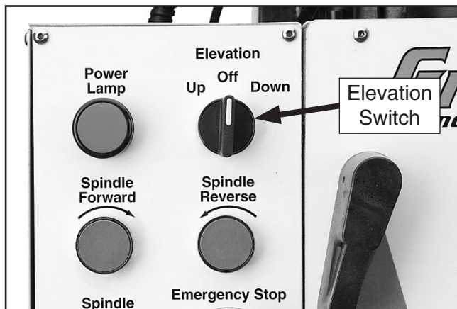
Figure 14. Elevation switch that controls motorized head travel.
