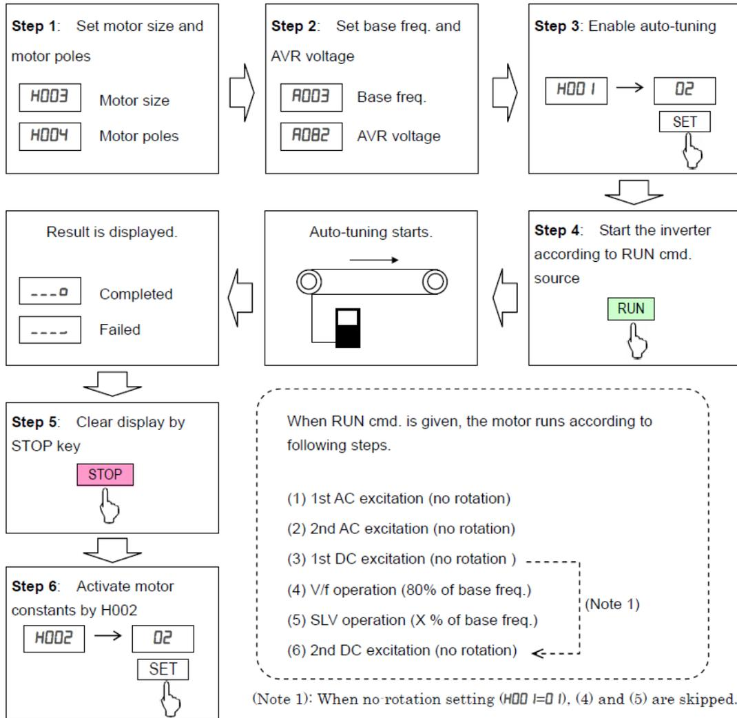
(Note 2) After auto tuning is completed, be sure to set 01 in H002/H202, otherwise measured data is not effective.
