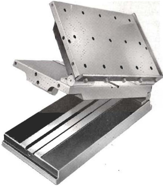
Fig. 36. Compound Sine Plate
