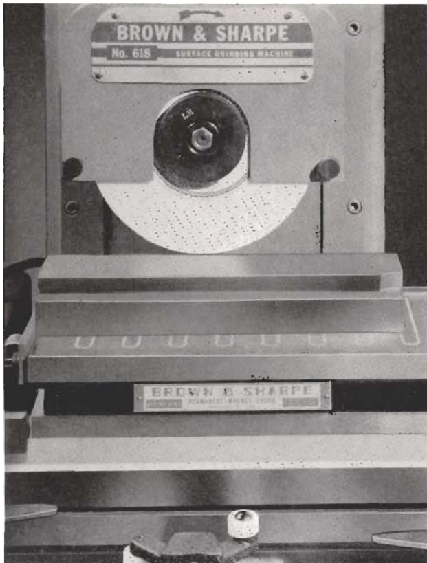
Fig. 13. Another typical operation in which slot and side wheel grinding are featured.
