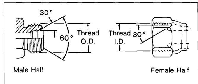
This connection is sometimes used in fluid power systems. The female half has a straight thread and an inverted 30° seat. The male half of the connection has a straight thread and a 30° internal chamfer. The seal takes place by compression of the 30° seat on the chamfer. The threads hold the connection mechanically.
