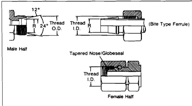
This connection consists of a common male and two different females. The Millimetrique Series is used with whole number metric O.D. tubing and the GAZ Series is used with fractional number metric O.D. pipe size tubing.
