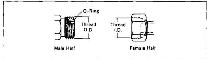
This connection offers the very best leakage control available today. The male connector has a straight thread and an O-Ring in the face. The female has a straight thread and a machined flat face. The seal takes place by compressing the O-Ring onto the flat face of the female, similar to the split flange type fitting. The threads hold the connection mechanically.
