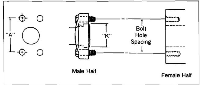
This connection is commonly used in fluid power systems. There are two pressure ratings. Code 61 is referred to as the "standard" series and Code 62 is the "6000 psi" series. The design concept for both series is the same, but the bolt hole spacing and flanged head diameters are larger for the higher pressure, Code 62 connection.
