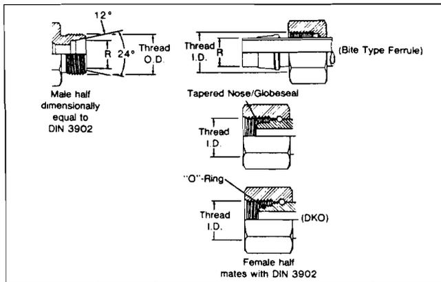
This connection style consists of a common male and three different female halves.
