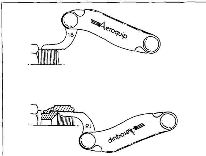
Use a thread pitch gauge to determine the number of threads per inch or the distance between threads in metric connections. Place the gauge on the threads until the fit is snug. Match the measurement to the charts.
