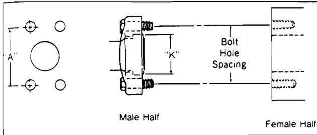
This connection is commonly used in fluid power systems. There are two pressure ratings. PN 35/350 bar (Code 61) is the "standard" series and PN 415 bar (Code 62) is the high pressure series. The design concept for both series is the same, but the bolt hole spacing and flanged head diameters are larger for the higher pressure, PN 415 bar connection. Both metric and inches bolts are used. The port will have an "M" stamped on it if metric bolts are required.
