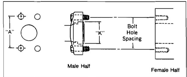
This connection is commonly used in fluid power systems. There are two pressure ratings. Form R (Code 61) is referred to as the "standard duty" series and Form S (Code 62) is the "heavy duty" series. The design concept for both series is the same, but the bolt hole spacing and flanged head diameters are larger for the higher pressure, Form S connection. Both metric and inch bolts are used.
