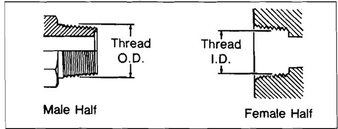
This BSPT (tapered) connection is similar to the NPT, except that the thread pitches are different in most sizes, and the thread form and O.D.s are close but not the same. Sealing is accomplished by thread distortion. A thread sealant is recommended.
