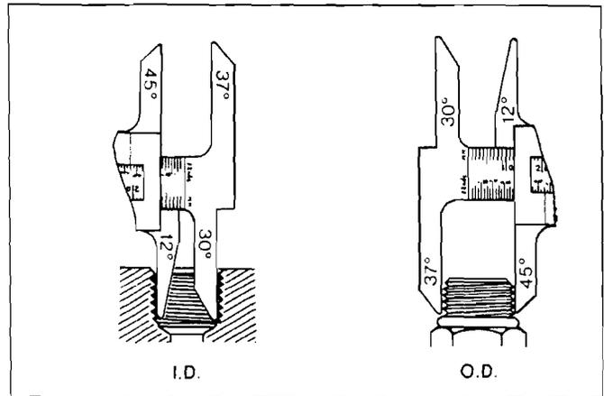
Measure the thread diameter with an I.D./O.D. caliper as shown. Match the measurements to the charts.
