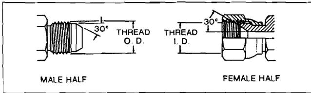
The Japanese JIS 30° flare is similar to the American SAE 37° flare connection in application as well as sealing principles. However, the flare angle and dimensions are different. The threads are similar to BSPP.
