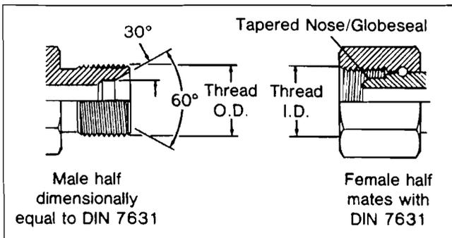
This connection is frequently used in hydraulic systems. The male has a straight metric thread and a 60° (included angle) recessed cone. The female has a straight thread and a tapered nose/Globeseal™ seat. The seal takes place by contact between the cone of the male and the nose of the tapered nose/Globeseal flareless swivel. The threads hold the connection mechanically.
