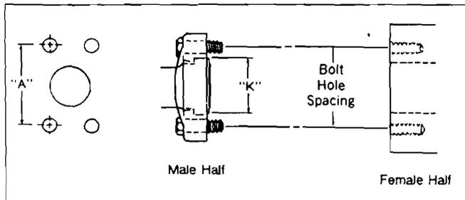
This connection is commonly used in fluid power systems. There are two pressure ratings. Type I (Code 61) is referred to as the "standard" series and Type II (Code 62) is the "6000 psi" series. The design concept for both series is the same, but the bolt hole spacing and flanged head diameters are larger for the higher pressure, Type II connection. Both metric and inch bolts are used.
