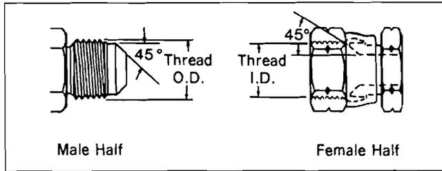
This connection is commonly used in refrigeration, automotive and truck piping systems. The connector is frequently made of brass. Both the male and female connectors have 45° seats. The seal takes place between the male flare the female cone seat. The threads hold the connection mechanically.
