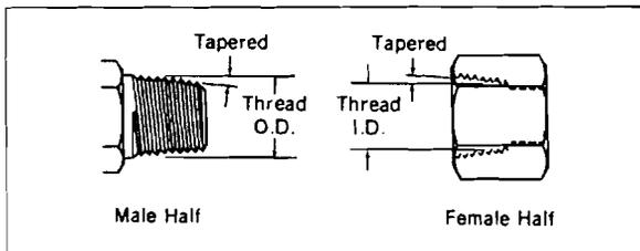
The JIS tapered thread is similar to the BSPT connection in design, appearance and dimensions. The JIS tapered thread and the BSPT connection are interchangeable.
