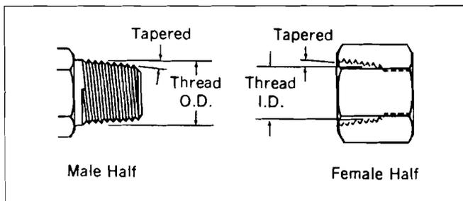
This connection is still widely used in fluid power systems, even though it is not recommended by the National Fluid Power Association (NFPA) for use in hydraulic applications. The thread is tapered and the seal takes place by deformation of the threads.
