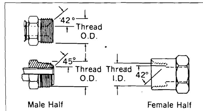
This connection is frequently used in automotive systems. The male connector can either be a 45° flare in the tube fitting form or a 42° seat in the machined adapter form. The female has a straight thread with a 42° inverted flare. The seal takes place on the flared surfaces. The threads hold the connection mechanically.
