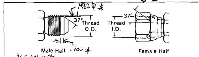
This connection is very common in fluid power systems. Both the male and female halves of the connections have 37° seats. The seal takes place by establishing a line contact between the male flare and the female cone seat. The threads hold the connection mechanically.
