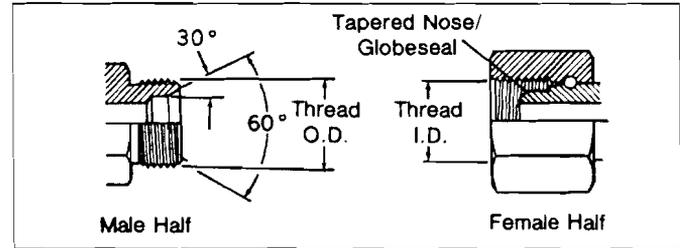
The BSP (parallel) male is similar to the NPSM male except the thread pitches are different in most sizes. The female swivel BSPP has a tapered nose/Globeseal flareless swivel which seals on the cone seat of the male.
