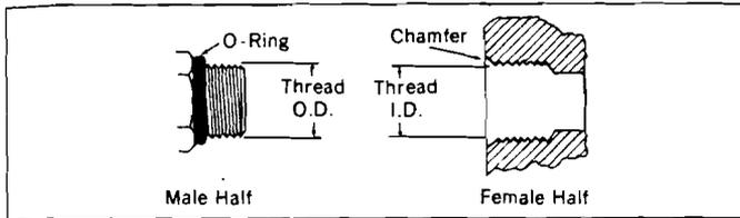
This port connection is recommended by the NFPA for optimum leakage control in medium and high pressure hydraulic systems. The male connector has a straight thread and an O-Ring. The female port has a straight thread, a machined surface (minimum spotface) and a chamfer to accept the O-Ring. The seal takes place by compressing the O-Ring into the chamfer. The threads hold the connection mechanically.
