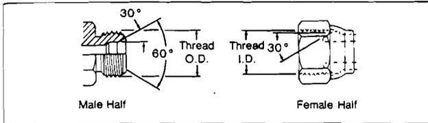
The JIS parallel is similar to the BSPP connection. The JIS parallel thread and the BSPP connection are interchangeable.
