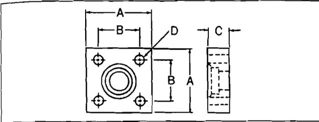
The JIS 4-Bolt square flange connection is similar in concept to the SAE 4-bolt flange connection, except that the JIS bolt pattern is square and the flange itself is different.
