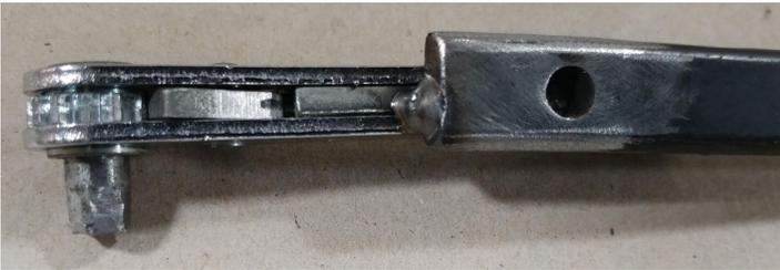
The extension rod I used was from a broken Irwin clamp, it was hardened and I did not want to destroy my band saw blade and I was too lazy to cut it with a grinder. The unused bad end is saved as a reminder of the sometimes shady quality of HF tools.
