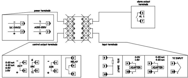
I think terminals #1 & #2 are for the line in power, either 110 or 12v dc. And terminals #4 & #5 are for the SSR module. Am I correct? So, I wire the MK 1 to the 24/-380 VAC side of the SSR and the input side of the SSR to terminals #4 & #5 respectively, correct. Please feel free to correct and augment this diagram as I don't want ruin any components and re spend money. Thank You.
