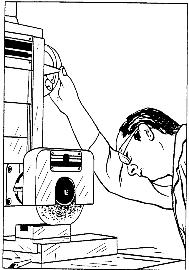
Fig. 3. The vertical adjustment hand wheel is shown near the top of the upright
