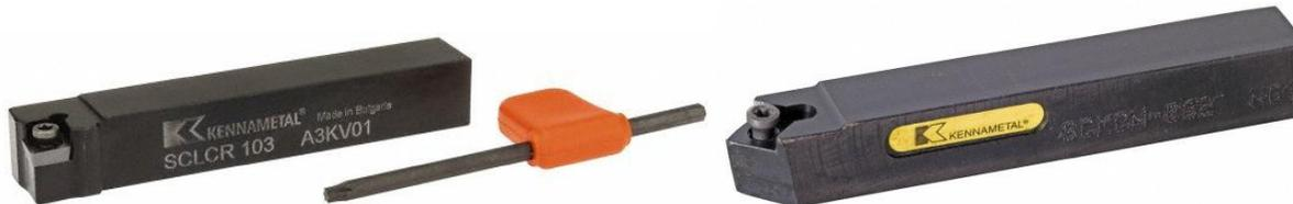
SDJC 55 Degree diamond neutral rake uses DC..32.5 Inserts such as DCMT or DCGT 32.51 or 32.52. This is a narrow profile insert, good for getting into tight (narrow) cutting areas, neutral works well for chamfering.
