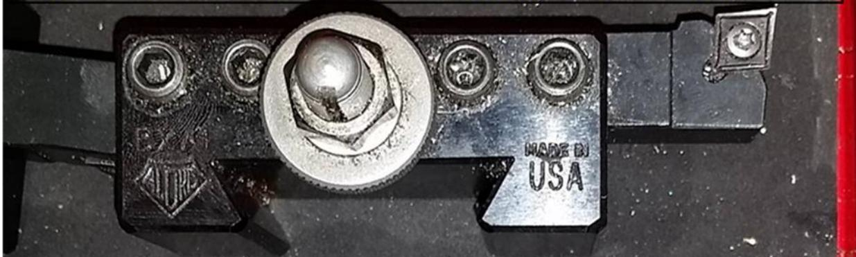
**Seco - MWLNR 10-3A Tool Holder uses WNMG 33.. inserts**
