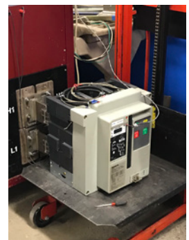
Primary Injection Testing
