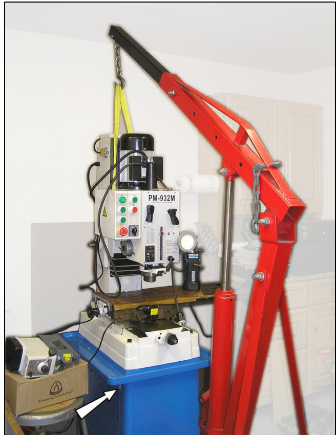
Figure 5-4 Lowering mill onto stand tray
