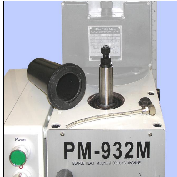
Figure 2-2 Spindle and drawbar
