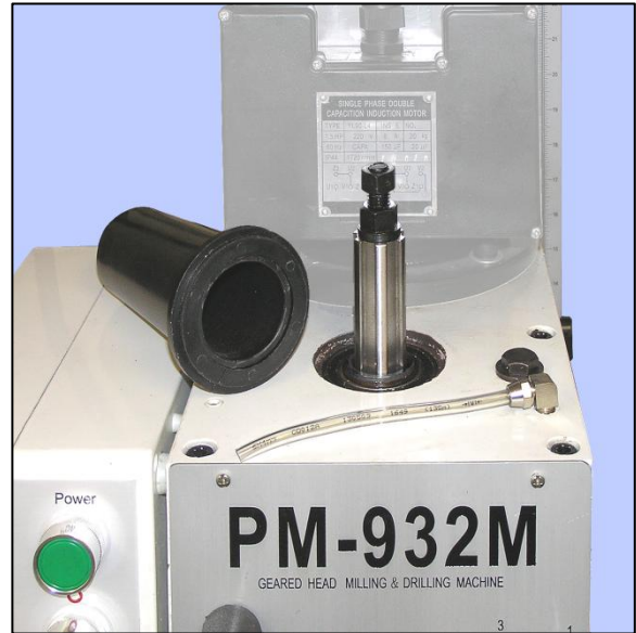
Figure 2-2 Spindle and drawbar
