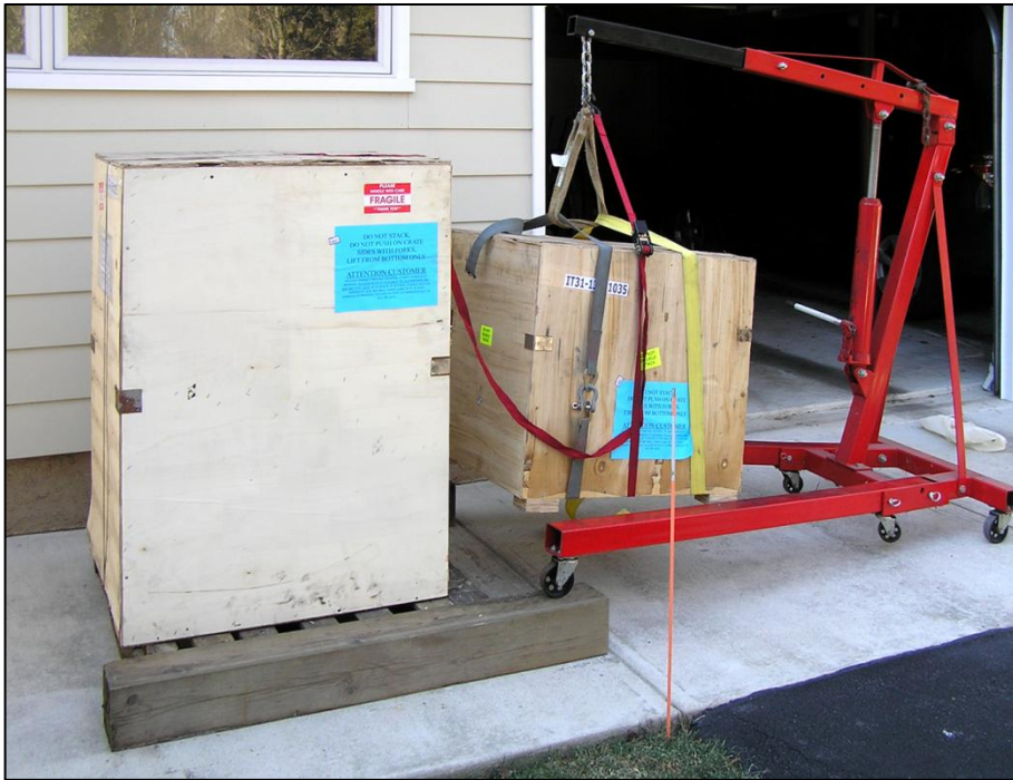
Figure 5-1 One method of removing the upper packing case
