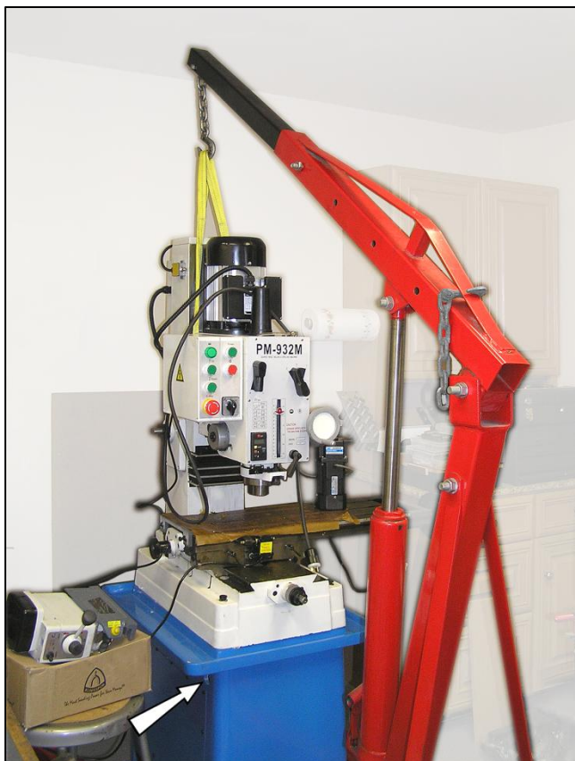
Figure 5-4 Lowering mill onto stand tray
