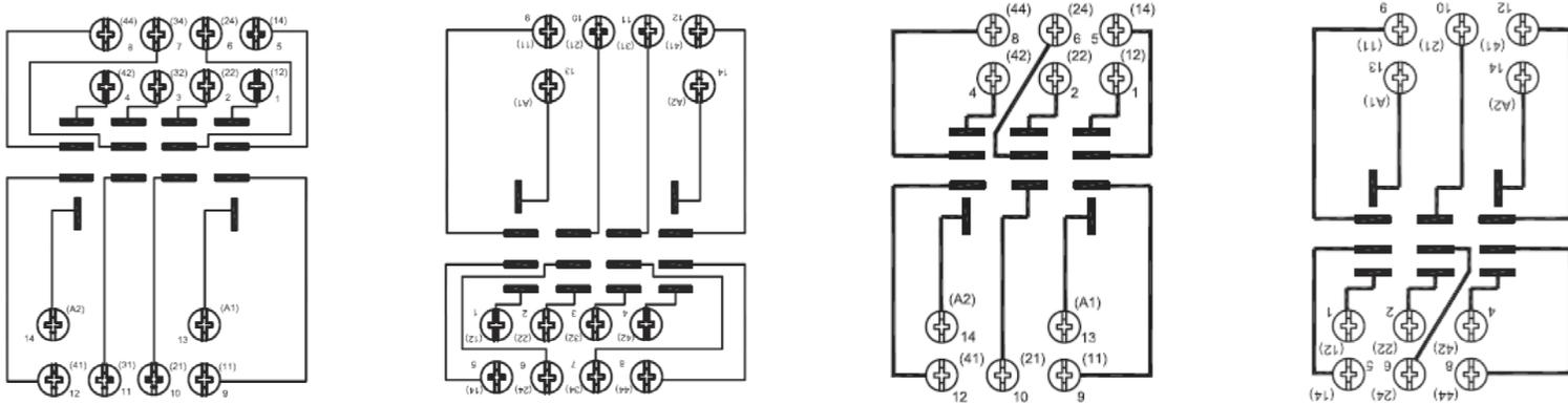
Note that relay connections in sockets is different then the relay, connect via the labeled numbers on the socket screw terminals. Note proper polarity and orientation of diodes and LEDs, the banded side is the (-) cathode
