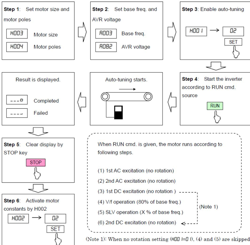
(Note 2) After auto tuning is completed, be sure to set 01 in H002/H202, otherwise measured data is not effective.
