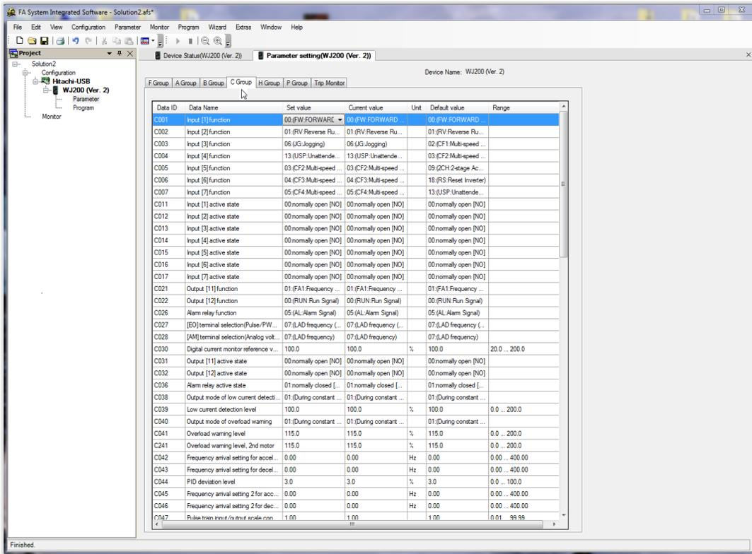
Motor Auto-tune determines your motors actual operating parameters, which can be entered in the VFD program variables
