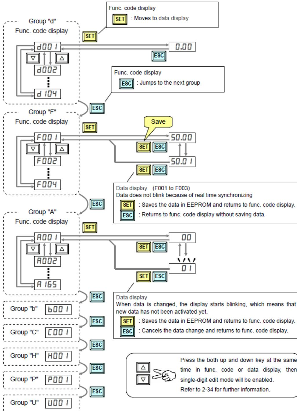
**NOTE:** Pressing the [ESC] key will make the display go to the top of next function group, regardless the display contents. (e.g. A02 1 → [ESC] → b00 1)
