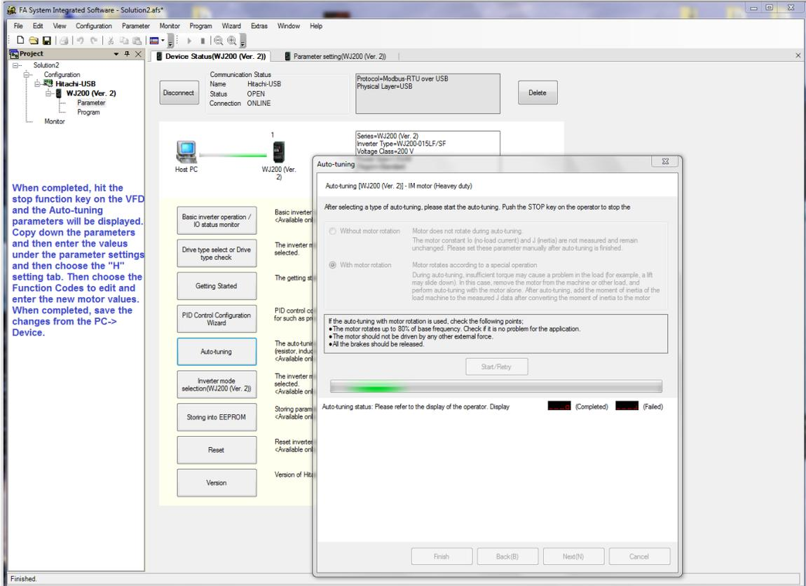
When completed, hit the stop function key on the VFD and the Auto-tuning parameters will be displayed. Copy down the parameters and then enter the values under the parameter settings and then choose the "H" setting tab. Then choose the Function Codes to edit and enter the new motor values. When completed, save the changes from the PC-> Device.
