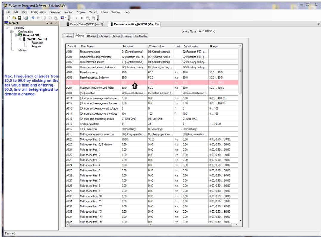
Program variable changes must be sent from the PC to the VFD, either Left click on the "Program" pull down menu tab, or Right click on the highlighted parameter to pull up the menu.
