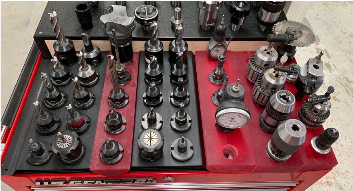
I find this Royal EasyChange setup very useful and preferable to my Maxi power drawbar for quick tool change sequences such as spot drill, drill, chamfer, and tapping in sequence as [illustrated here](#). I do swap back and forth between the EasyChange system and using a conventional drawbar for more aggressive tooling such as indexable end mills, face mills, and heavy boring head operations.
