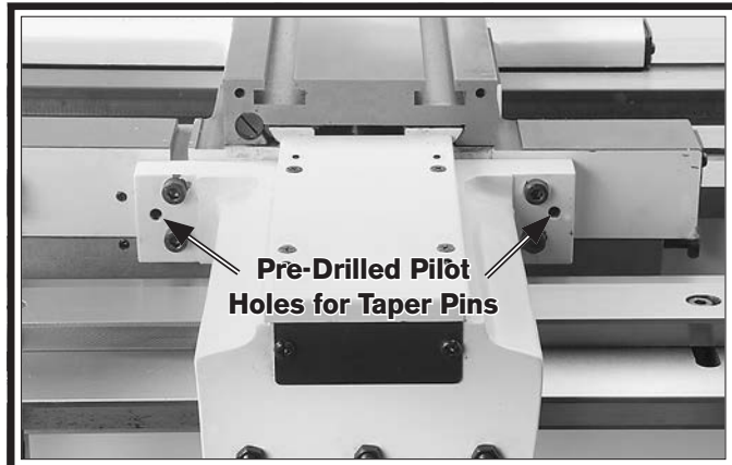
Figure 23. Taper pin pilot holes.
